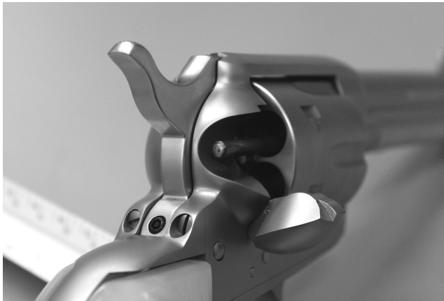
Figure 4.6 Solid frame revolver with spring-loaded ejector rod depressed. The loading gate is open. (Image from author's collection.)
